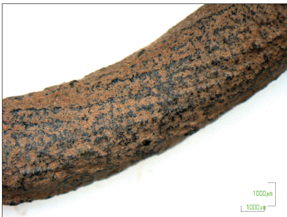
Fig. 8. Microscopic photo of traces of wire drawing on draw plate (image by K. Żołędziowski).
