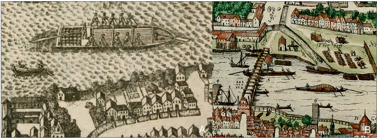
Fig. 2. A – pictorial representation of the Oder vessel, so-called Schale , with broad hull and flat, transom aft. Detail of the Alten Stettin , created by Heinrich Kote in 1625 (Copyright: Archiwum Państwowe w Szczecinie / signature: PL-65-46-0-357); B – elongated vessels on the Oder River can be associated with the early Kahn -type. Detail of the coloured edition of Alten Stettin published in Civitates orbis terrarum , vol. IV by Georg Braun and Frans Hogenberg, circa 1600 (Public domain).
