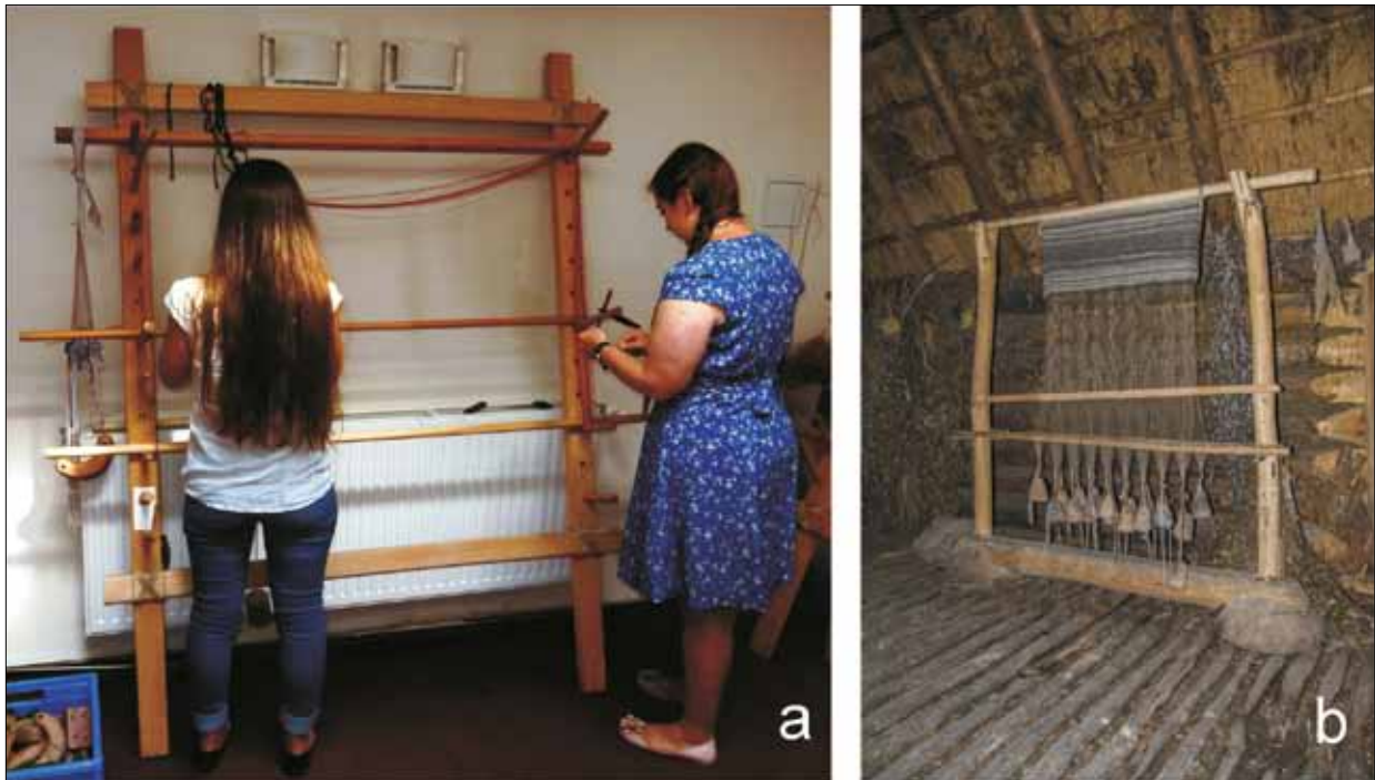
Fig. 1. Two types of warp-weighted looms of modern construction: a) the Scandinavian type used in the Institute of Archaeology, University of Warsaw (photo by the author), b) the free standing type used in the Biskupin Archaeological Museum (photo by Łukasz Gackowski).
