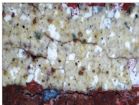
Fig. 5. Semi-transparent, yellowed layer covering the white paint layer, visible in the micro-photograph of the strip above the uraeus frieze (PCMA UW | photo P. Staszkieicz)
