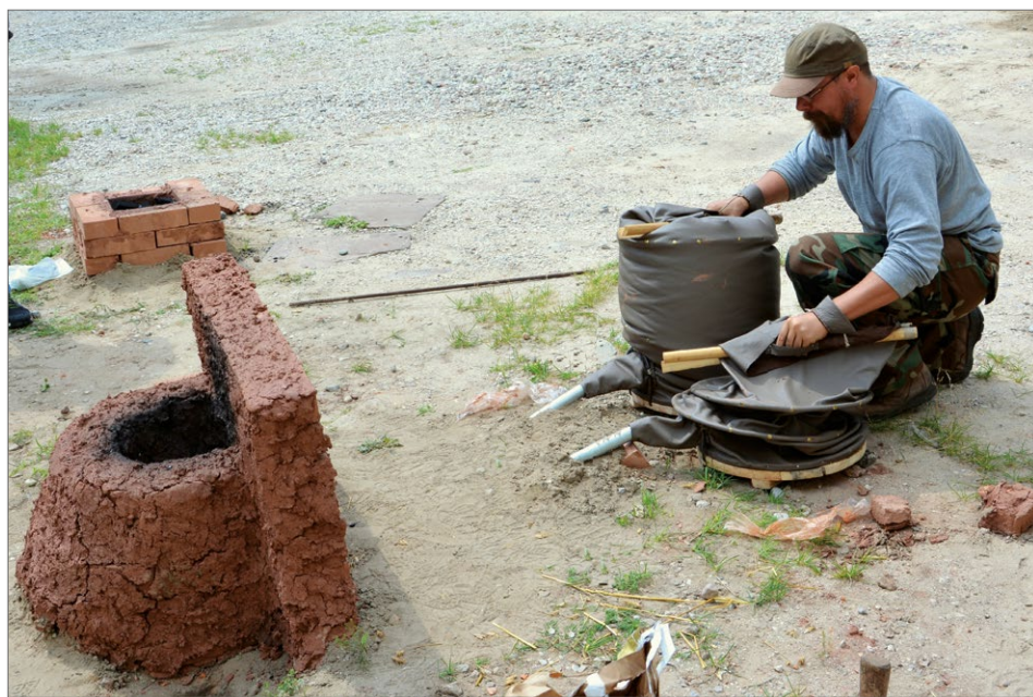
Fig. 8. First stage of the melting process: furnace and bellows; note the pipes from the bellows supplying air to the hearth (Photo J. Rądkowska)
