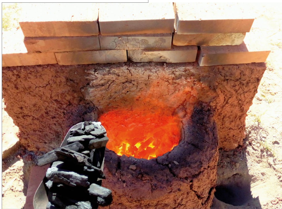
Fig. 9. Second stage of the melting process: top, the screen wall protecting from the heat is higher now; bottom, stoking the hearth with coal from the top (Photos J. Rądkowska)
