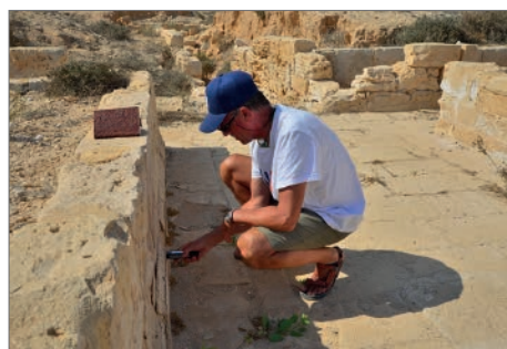
Fig. 1. Dampness study: left, thermovision measurements in the main square of the ancient town; right, wall humidity measurements being taken in Tomb T21 (Polish-Egyptian Conservation Mission | thermovision-image processing P. Zambrzycki, photo A. Selerowicz)
