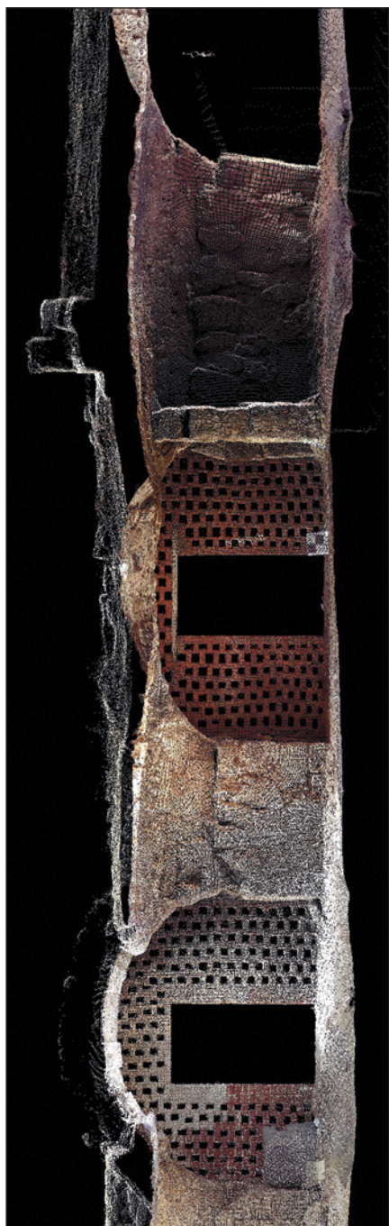
Fig. 9. Photogrammetric scan of the underground vaulted structure, western wing (Processing W. Terlikowski, P. Bartosiak)
