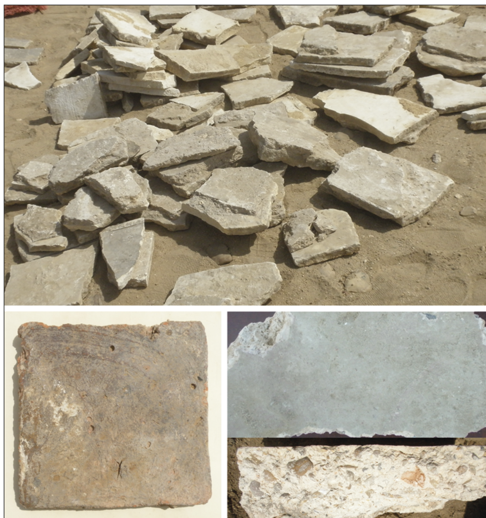
Fig. 9. Floor tiles from the rubble of D.50: top, assorted tiles of nummulithic limestone; left, ceramic tile, top view; right, piece of lime mortar floor with section view (not to scale)
