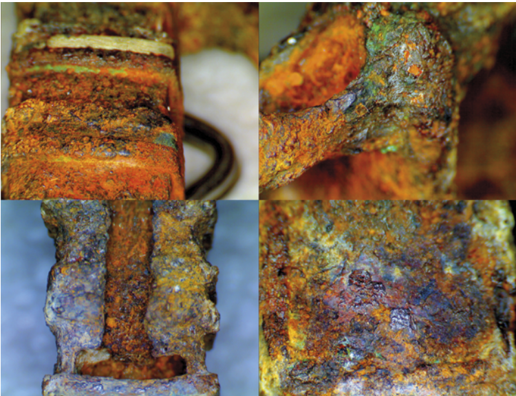
Fig. 16. Lock or padlock; microscopic photos: top left, rear view of lock section; top right, lock slot and tongue; bottom right, traces of copper oxides near metopes; bottom left, traces of copper oxides near the bow/rail section
